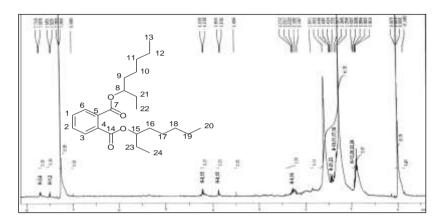
Figure 15 <sup>1</sup>H NMR spectrum of isolated compound MM-3 (400 MHz, CDCl<sub>3</sub>)
