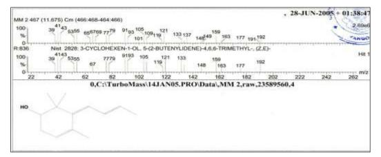
**Figure 12** GC-MS spectrum of MM-2 compared with that of 3-cyclohexen-1-ol, 5-(2-butenylidene)-4, 6, 6-trimethyl-,(Z,E) from GC-MS library data
