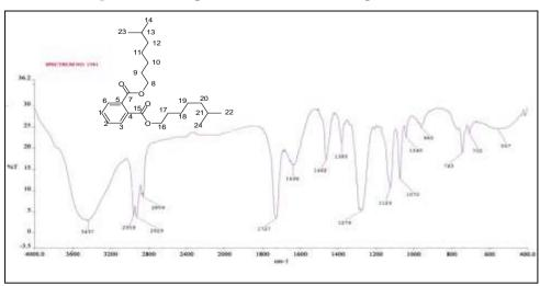
Figure 6 FT-IR spectrum of isolated compound MM-1
