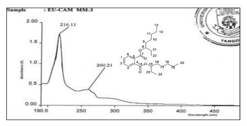
Figure 13 UV spectrum of isolated compound MM-3
