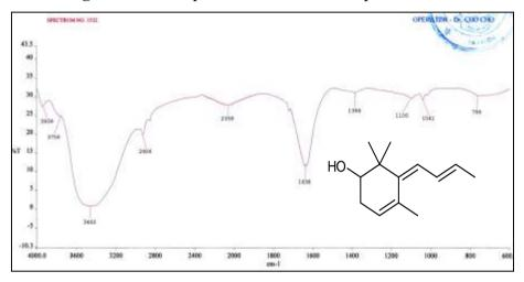
Figure 11 FT-IR spectrum of isolated compound MM-2 (KBr)
