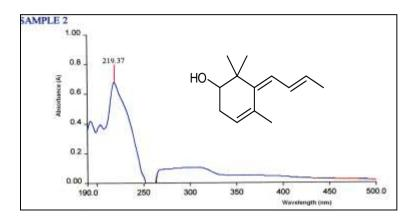
Figure 10 UV spectrum of isolated compound MM-2
