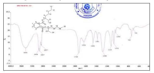
**Figure 14** FT-IR spectrum of isolated compound MM-3 (KBr)
